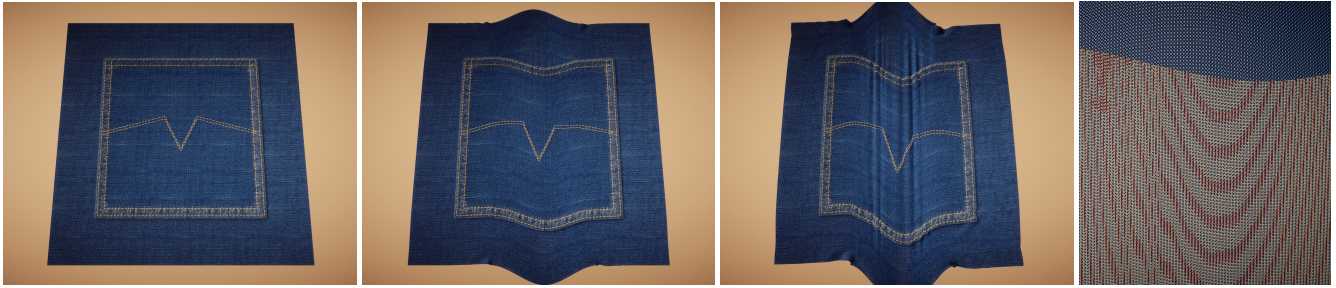
Fig. 5. Snapshots of a simulation of a jeans back pocket. The scene consists of two layers of yarn-level twill denim fabric, stitched on the sides and at the bottom. We pull from the top and the bottom, inducing sliding of the two layers, as well as wrinkles influenced by the combined material. The full simulation is resolved with implicit contact handling in our EoL formulation, and it has over 645K nodes. When the layers slide, the two groups of sliding warp and weft yarns induce pervasive degeneracies in the discretization. The rightmost image shows the soup of nodes at the top of the pocket, with EIL nodes in red.
